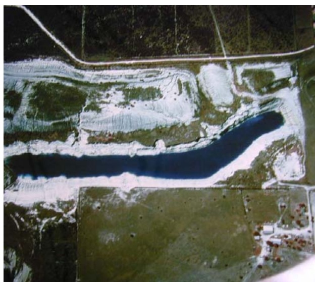
Figure 10: Aerial photo of the Weddington Open Pit in 1988. This mine was initiated in 1972 and was restored in 1999. Note the eroding spoil piles. The pit lake is approximately 3000 feet long. Source: RRC
